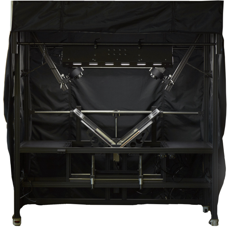
BC100 shown with two DT RCam Reprographic Cameras using 40 megapixel high resolution digital backs.
